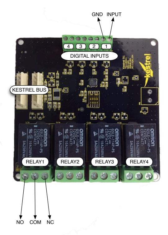
NO: Normally Open Connection COM: Common Connection NC: Normally Closed Connection
